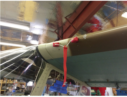
Siai Marchetti 1019 Ventilation Scoop Plugs ENGINE PLUGS PREVENT BIRD NEST FOD. Piper Saratoga Engine Cowling Bird's Nest
