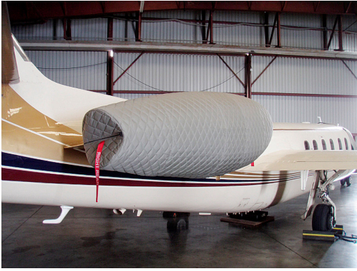
IAI Westwind 1124 Insulated Engine Nacelle Cover
