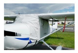
Cessna 150 & 152 Extended Canopy Cover (Over-Top, Down To Fuselage, Extends To Cover Gas Caps)
