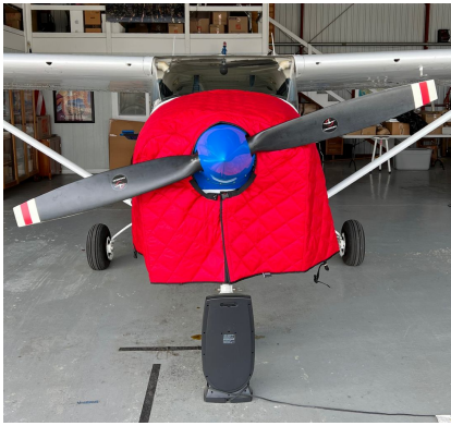
Insulated Hangar Blanket on Cessna 182
