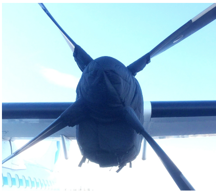
ATR-72-202 Insulated Engine & Prop Hub Covers
