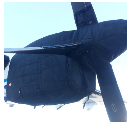
ATR-72-202 Insulated Engine & Prop Hub Covers
