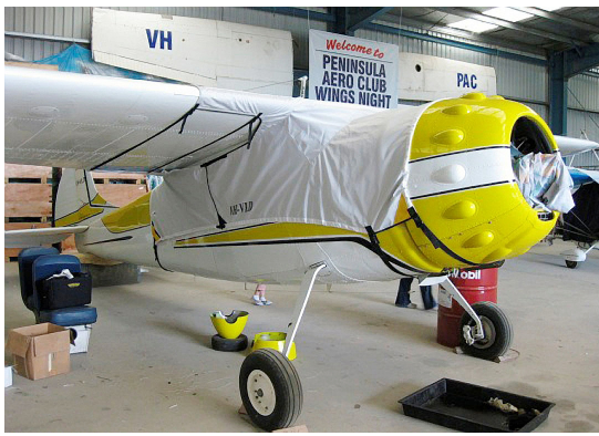
Cessna 195 Canopy Cover, over-top, 24" fwd ext to cover cowl ring gap, gas cap ext.
