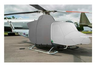
Bell 412 Forward Cabin/Nose, Insulated Engine, Tailboom, Rotor Hub Forward Cabin Nose & Mid-Cabin/Engine Cover (extended & Blade Covers to cross tubes)
