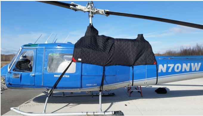
Bell 204 Insulated Engine Area Cover
