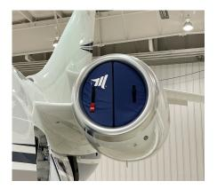
Falcon Jet Engine Inlet Plugs Folding Type
