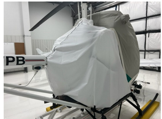
Schweizer 300C Engine Cover, test fit cover
