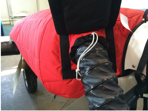
Cessna 402 Insulated Engine Cover with Heater
