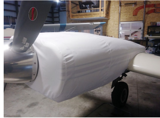
Cessna 310B Engine Covers, test fit cover
