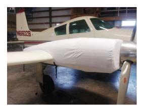
Cessna 310B Engine Covers, test fit cover
