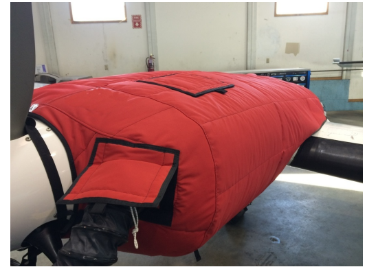
Cessna 402 Insulated Engine Cover with Heater
