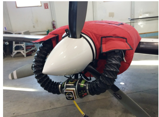
Cessna 402 Insulated Engine Cover with Heater
