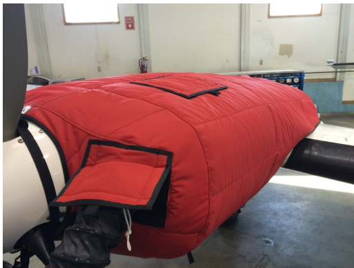
Cessna 402 Insulated Engine Cover with Heater
