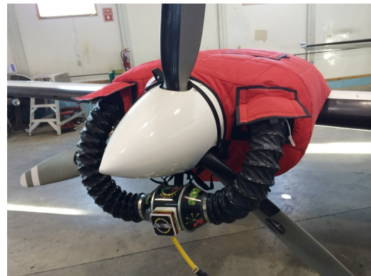
Cessna 402 Insulated Engine Cover with Heater
