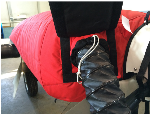
Cessna 402 Insulated Engine Cover with Heater
