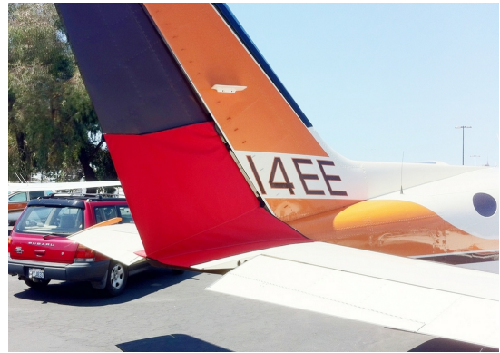
Cessna 414 Rudder Openings Cover (bird barrier)
