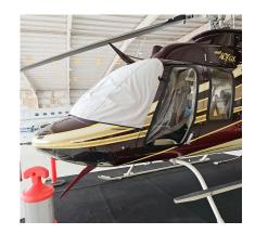
JetRanger Bubble, Engine, Rotor Hub & Blade Covers (& Tie-Downs)
