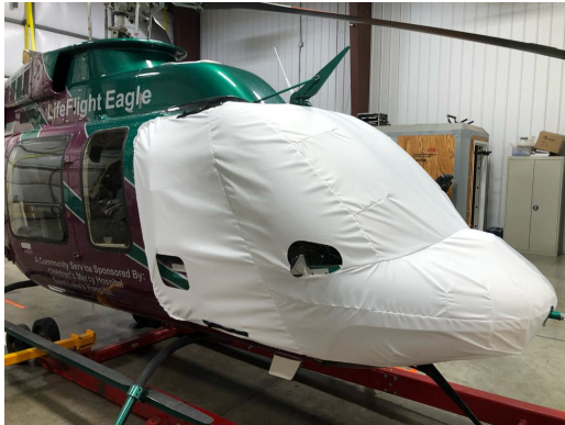
Bell 407 Abbreviated Bubble Cover, secures to doors, test fit cover
