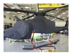
Bell 412 Cockpit/Canopy/Nose, Insulated Engine Area, Rotor Hub, Blade, Tailboom and Tail Rotor Coversroto
