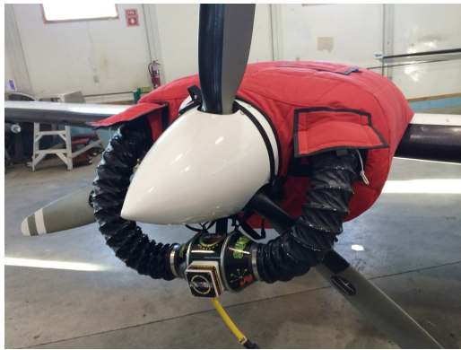
Cessna 402 Insulated Engine Cover with Heater
