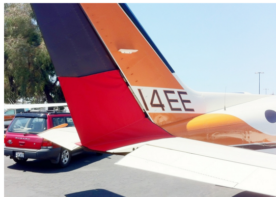
Cessna 414 Rudder Openings Cover (bird barrier)
