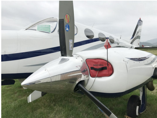
Cessna 340 Engine Inlet Plugs
