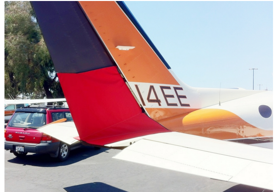
Cessna 414 Rudder Openings Cover (bird barrier)
