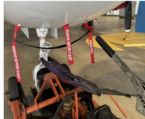
Cessna 421C Pitot Covers, Nose Inlet Plug
