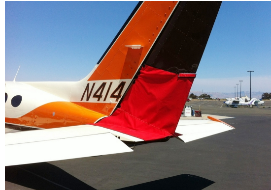
Cessna 414 Rudder Openings Cover (bird barrier)
