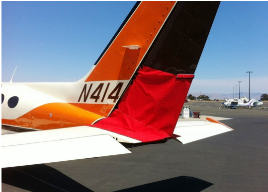
Cessna 414 Rudder Openings Cover (bird barrier)
