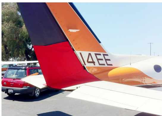
Cessna 414 Rudder Openings Cover (bird barrier)
