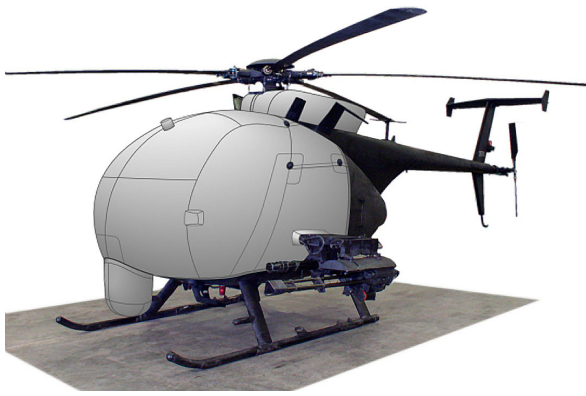
MH-6J Bubble, Flir & Doghouse Covers (illustration)
