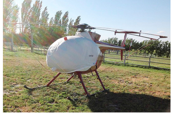
MD500D Bubble Cover with Intake Add-On
