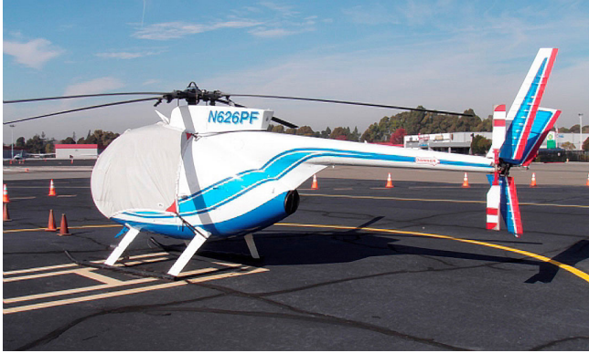
MD500C Bubble Cover with Wire Strike detail
