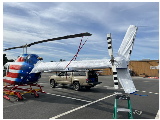
Bell 505 Tailboom & Stabilizer Covers, test fit cover
