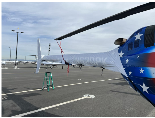
Bell 505 Tailboom & Stabilizer Covers, test fit cover
