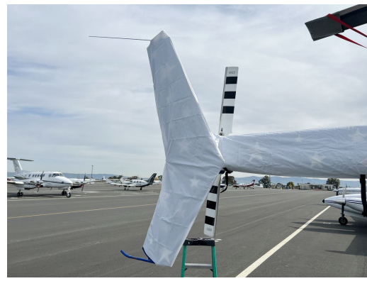
Bell 505 Tailboom & Stabilizer Covers, test fit cover
