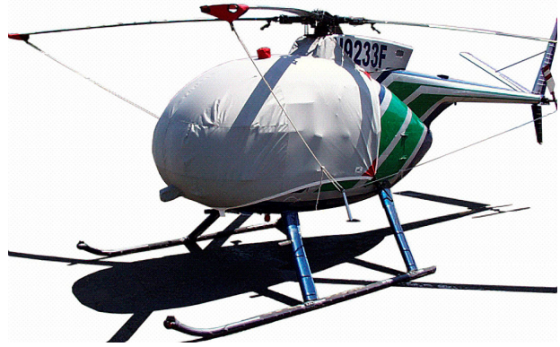
Hughes 500C Bubble Cover with Intake Add-on, Blade Tie-downs
