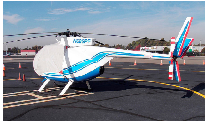
MD500C Bubble Cover with Wire Strike detail
