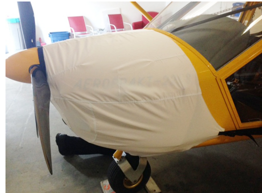
A-22 Engine Cover, test fit
