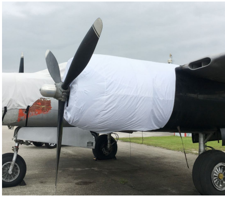
Douglas A-26 Engine Cover, test fit cover
