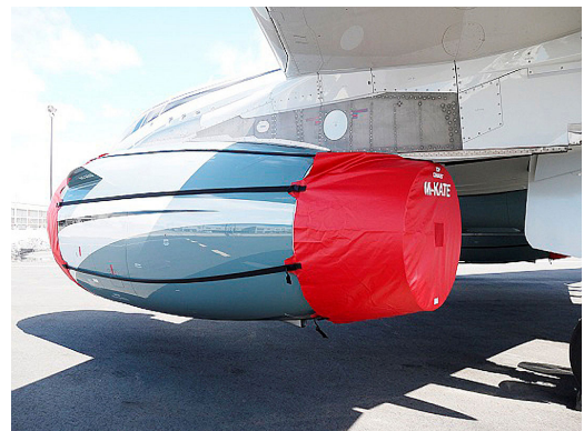
Airbus A319 Intake/Exhaust Covers set, IAE V2500
