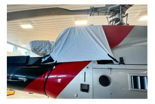
Airbus Helicopter H350 Bubble/Rotor Mast, & Intake Covers
