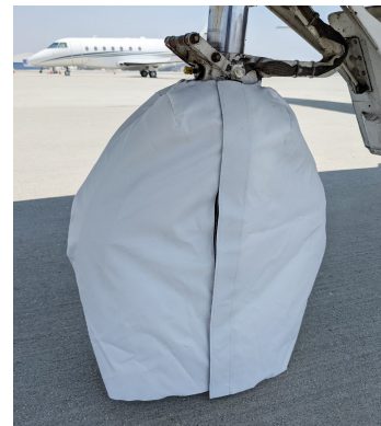
CJ1 Nose Gear Tire Cover, test fit
