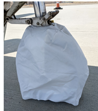
CJ1 Nose Gear Tire Cover, test fit
