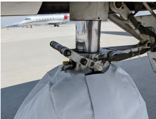
CJ1 Nose Gear Tire Cover, test fit
