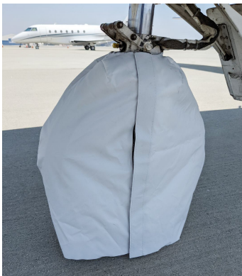
CJ1 Nose Gear Tire Cover, test fit
