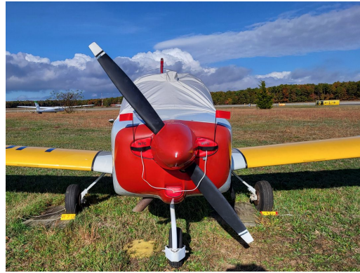
Grumman AA-1A Lynx Engine Inlet Plugs
