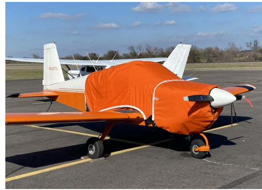
AA-1 Extended Canopy & Fully Enclosed Engine Cover
