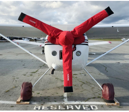
Cessna Skywagon Propellor/Spinner Cover, 3-blade type
