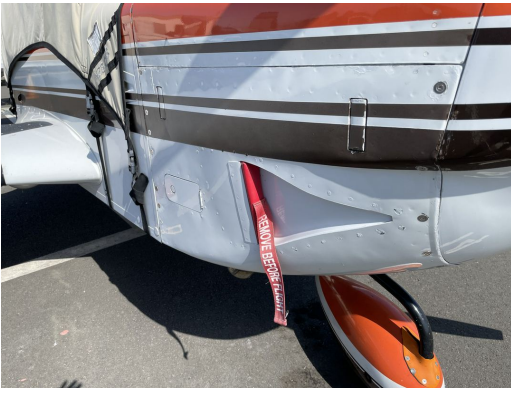
Grumman AA5 Side Cowling Inlet Plug
