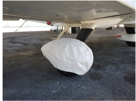
Grumman AA5 Main Wheelpant Cover, test fit
