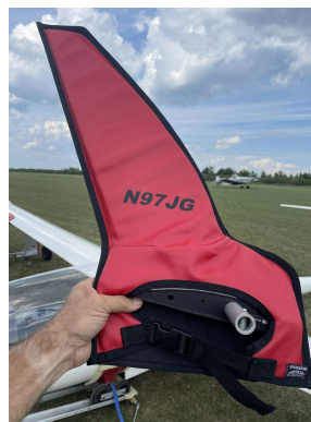
Schempp-Hirth Ventus-2B winglet/wingtip pads
