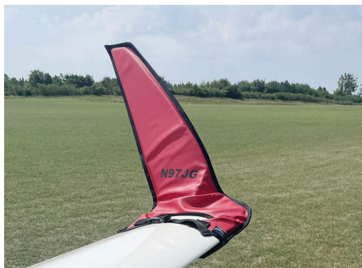
Schempp-Hirth Ventus-2B winglet/wingtip pads
