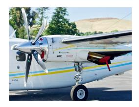
Aero Commander 690B Engine Inlet & Exhaust Plugs
