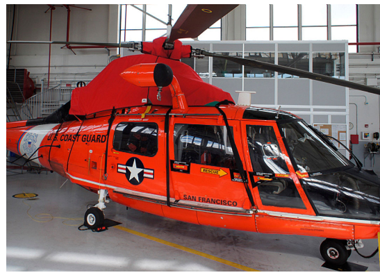
MH-65C Engine Area Cover, Swash Plate Aperture, Rotor Hub cover set, P/N: A365-210
