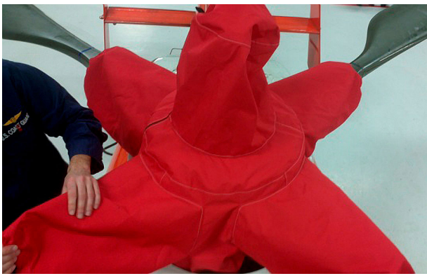
MH-65C Rotor Hub Cover w/ OADS Tube Cover detail
