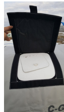
Alarus CH-2000 Insulated Engine Cover
