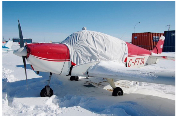
Alarus CH2000 Canopy Cover & Engine Plugs
