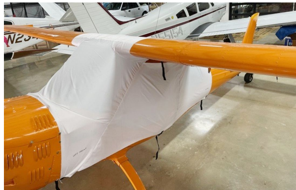
Aeromarine Merlin Over-Top Canopy Cover, test fit cover
