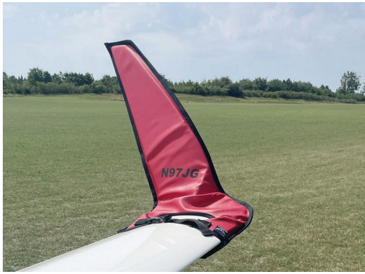
Schempp-Hirth Ventus-2B winglet/wingtip pads
