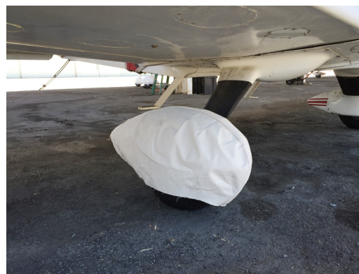
Grumman AA5 Main Wheelpant Cover, test fit
