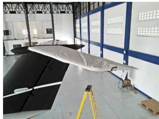
Beech King Air B350 Horizontal Stabilizer Covers
