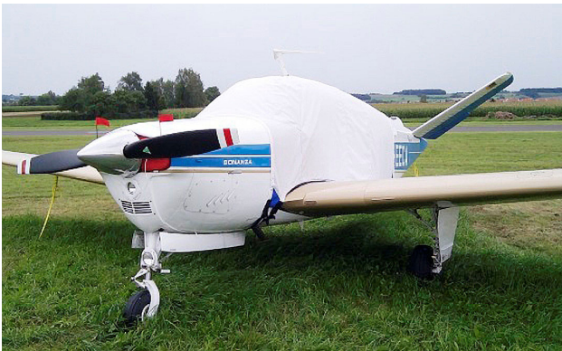
Bonanza Extended Canopy Cover & Engine Inlet Plugs Beech Bonanza/Debonair Extended Canopy Cover (With a Smiley Face)
