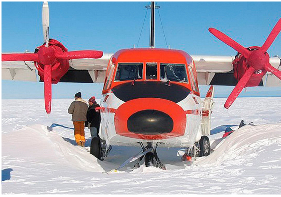
Casa 212 Insulated Engine & Propellor/Spinner Covers
