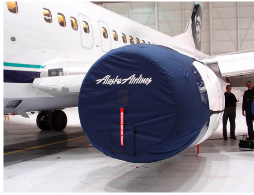
Boeing 737 Intake Covers with w/ Pre-heating hose access vent & attachment detail
