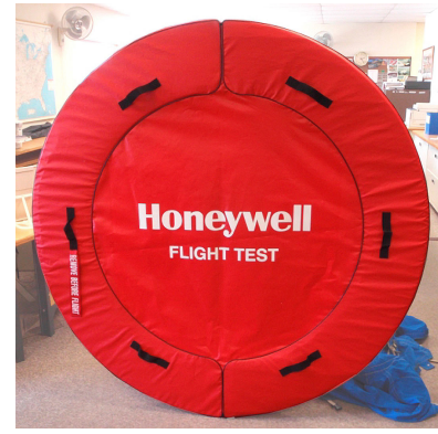
Boeing 757 Engine Intake Plugs, folding type
