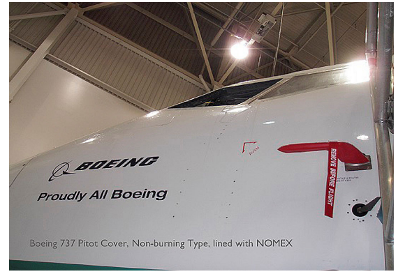
Boeing 737 Heat Resistant Pitot Cover
