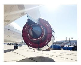
Boeing 787 Dreamliner Bypass Vent, Turbine Exhaust, & Exhaust Nozzle Plugs, Genx Engines
