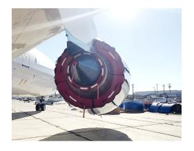
Airbus A330 Intake Plug, framed bi-fold type
