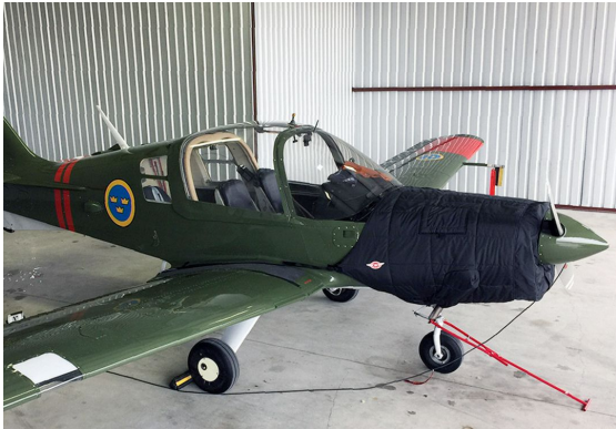
Scottish Aviation Bulldog Insulated Engine Cover
