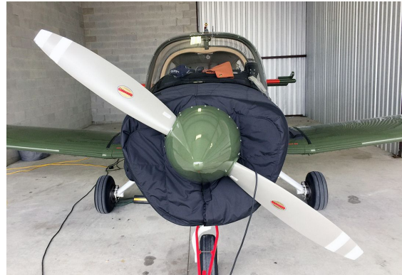
Scottish Aviation Bulldog Insulated Engine Cover
