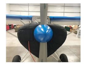
Bearhawk Patrol Insulated Engine Cover, with electric heater access flap
