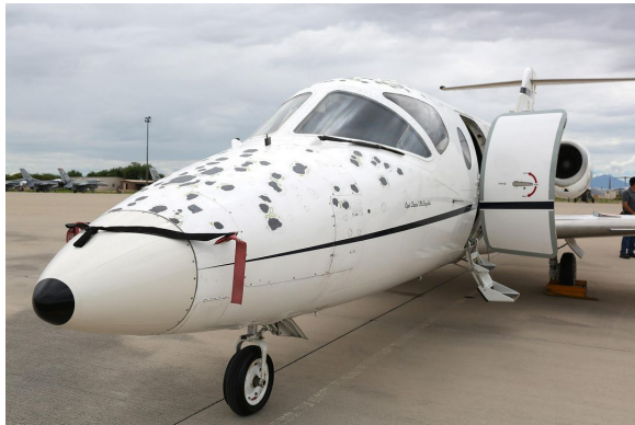
Raytheon Beechjet Hail Damage, and Pitot Covers
