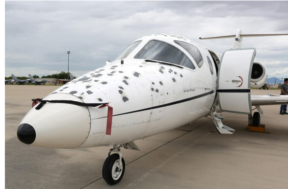
Raytheon Beechjet Hail Damage, and Pitot Covers
