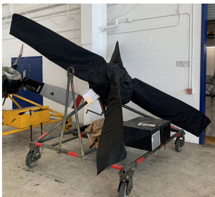
Lockheed C-130 Prop Cover, without spinner
