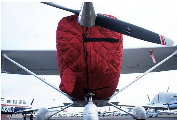
Cessna 172 Insulated Engine Cover, fully enclosed around bottom
